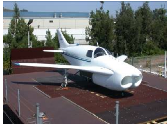
Figure 2. The DP-1 aircraft on the elevated test stand (tethers removed).
