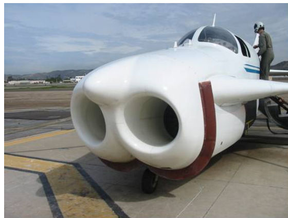
Figure 13. DP-1 with 5 inch cowl fence
