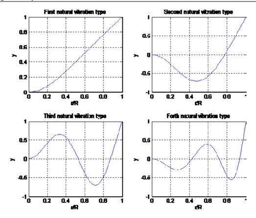
Figure 4.6 First Four Mode Shape of Non-rotating Blade
