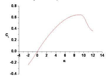
Figure 4.2 Lift Curve of Elliptical Airfoil
