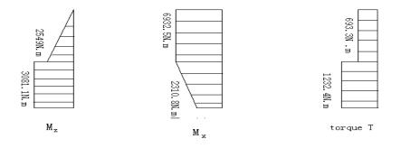
Figure 7.4 Bending Moment and Torque of Pillar
