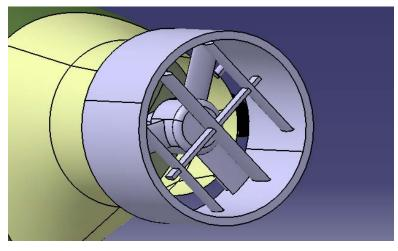
Figure 6.6 Vectored Thrust Ducted Propeller
