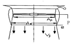
Figure 6.1 Vertical Ducted Propeller Sketch
