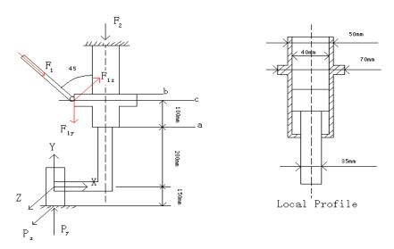
Figure 7.3 Size of Landing Gear and Force Analysis
