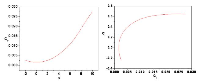
Figure 4.3 Drag Curve of Elliptical Airfoil
