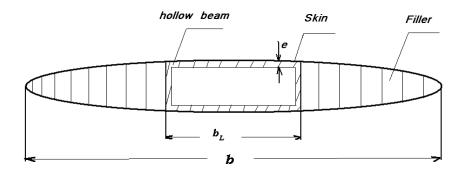
Figure 4.5 Cross Section of Blade
