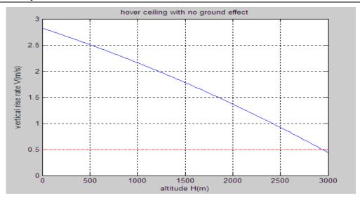
Figure 8.1 Hover Ceiling without Ground Effect
