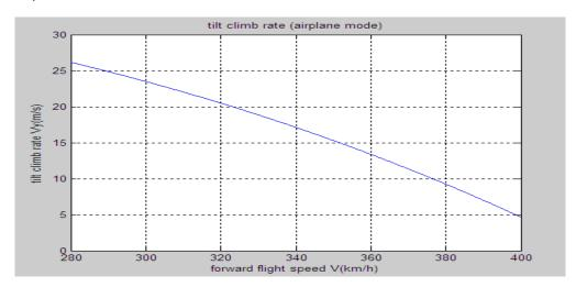
Figure 8.10 Tilt Climb Rate in Airplane Flight Mode
