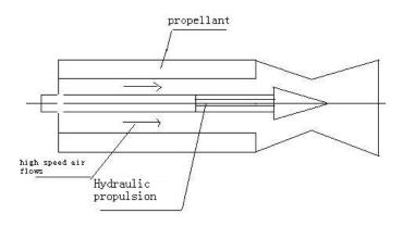
Figure 5.4 Variable Throat Area Engine Structure Sketch
