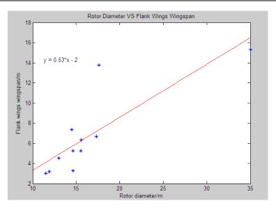
Figure 3.1 Rotor Diameter VS Flank Wingspan
