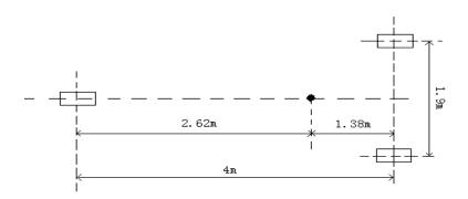
Figure 7.2 Size of Landing Gear
