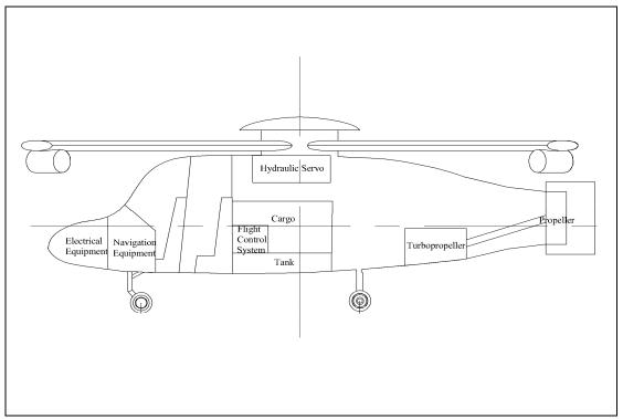
Figure 3.4 Arrangement for Helicopter
