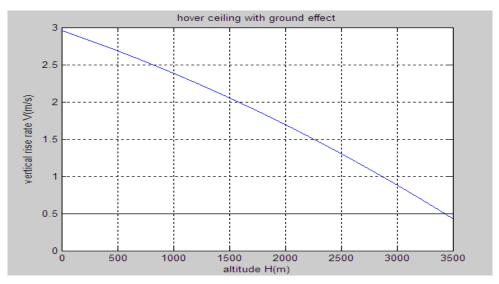
Figure 8.2 Hover Ceiling with Ground Effect
