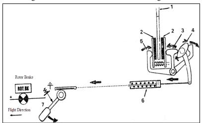
Figure 4.10 Rotor Brake of "Dolphin" Helicopter
