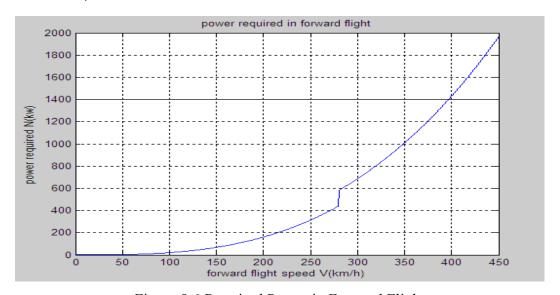
Figure 8.6 Required Power in Forward Flight
