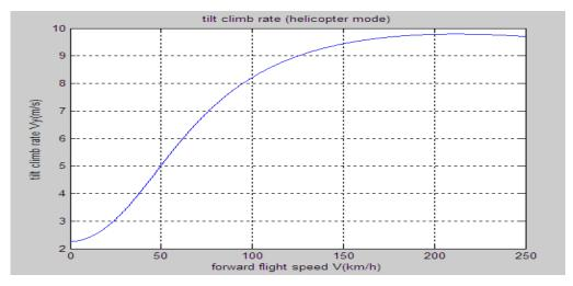
Figure 8.9 Tilt Climb Rate in Helicopter Flight Mode
