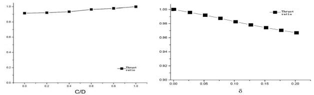
Figure 6.4 Effect of Duct Length on Thrust Ratio Figure 6.5 Effect of Tip Gap on Thrust Ratio
